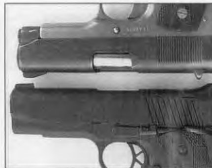
The Kimber's slide (bottom) is slightly longer than that of the Colt OM (top). Just enough so that the slide travel and cycle interval are increased to significantly enhance the operating reliability.
